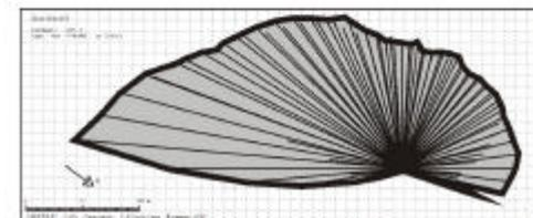
**Figure 3.** Cross-section made by laser scans. Two oblique planes. When rotated to overlap, the projection is parallel with the passage.
