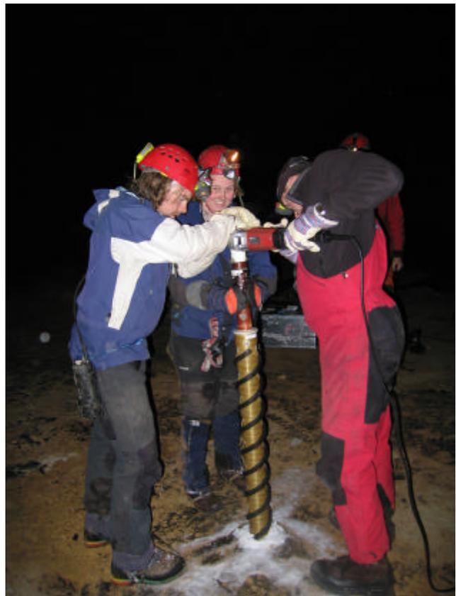
**Figure 9.** Drilling the ice core. Photo: S.E. Lauritzen
