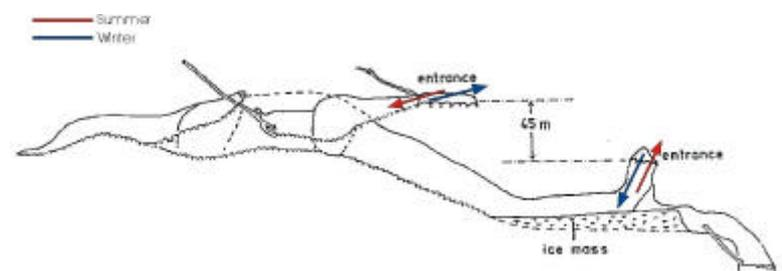
**Figure 4 (top).** Centerline map rotated until maximum overlap. In this case, the axis of projection is parallel with the general fold axis in the rock mass, demonstrating that the cave is indeed controlled by a major fold structure.
